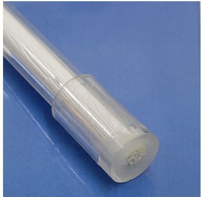
Fig16: A prototype. A bundle of hollow fibers fixed in a plastic tube.
