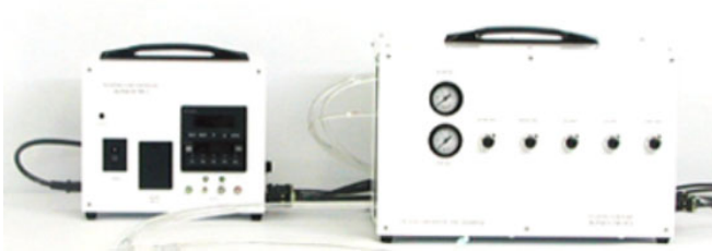
Fig2: A pump system for both steady flow and pulsating flow.
