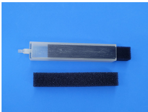
Fig.8: Cut plastic sponge and case with tube made with 3D printer.
