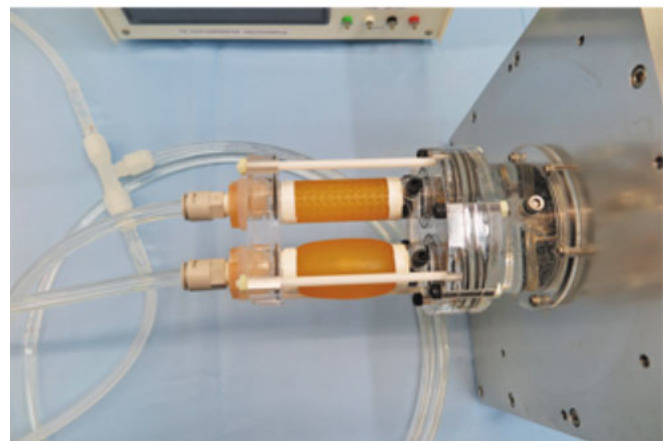
Fig. 1: A closed flow circuit type pulsating pump
